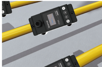
Fuel flow measurement
