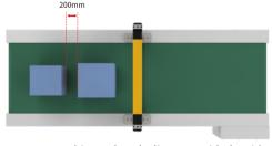
♦ The measuring system cannot measure objects placed adjacent or side-by-side.
